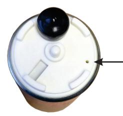
During installation ensure to check and eliminate any blockage or restrictions of the vapor-purge port. Failure to do so may cause your fuel pump to have slow or no priming which may lead to the damaging of your fuel pump.
