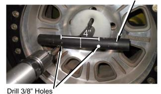
**c.** Double check the measurements of the marks and drill each hole out to 3/8".
