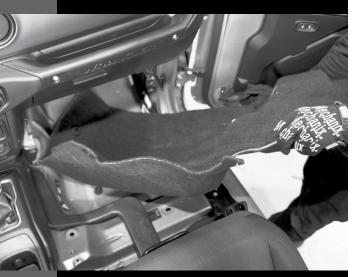
Remove factory plugs (2 front, 2 rear). The factory carpet from the cargo area should overlap the Armorlite flooring on the waterfall under the rear bench seat.
