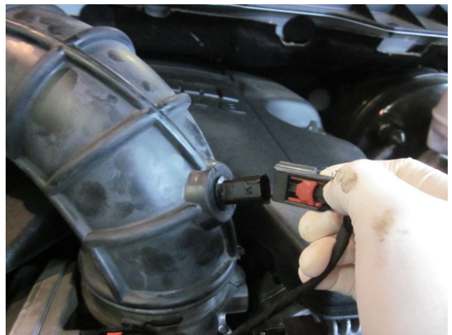
b) Disconnect the IAT (intake air temperature) sensor electrical connector from the sensor. Leave the sensor in place.
