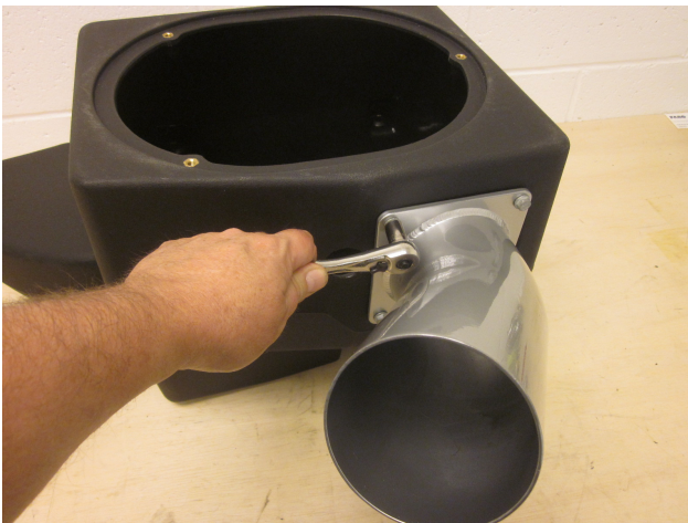
c) Attach the flanged air filter adaptor tube to the MOPAR Cold Air Box with four (4) M6 bolts provided. Pay attention to the adaptor tube's orientation with reference to the cold air duct.
