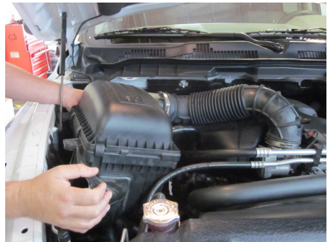
f) Pull up on the air box to disengage it from the locator pins and remove it from the engine compartment along with the intake hose.
