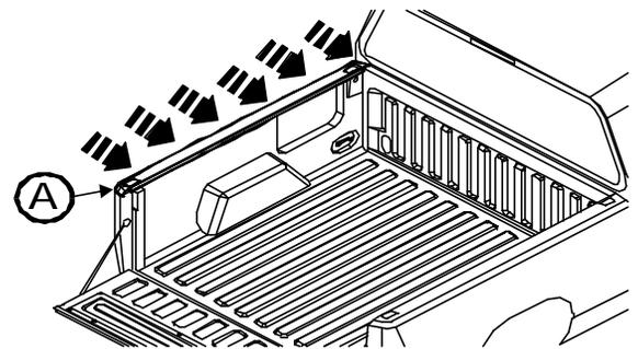
Note: If your side bedcap (A) has hardware enclosed, see Step 2 or Step 3 to complete your installation.
