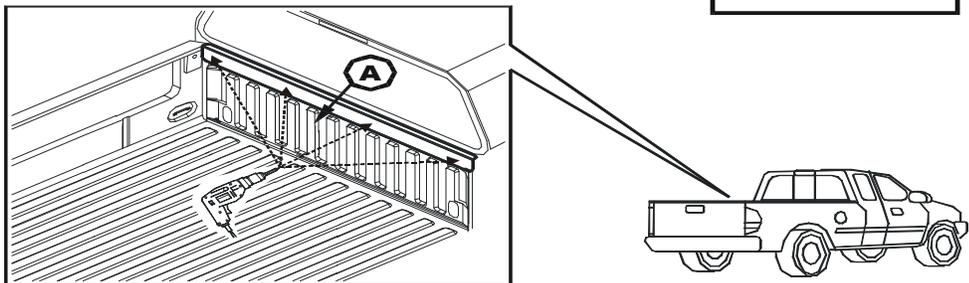
**3** Secure the front bed cap (A) into place by using the provided #8 x 1/2" phillips head screws (B).
