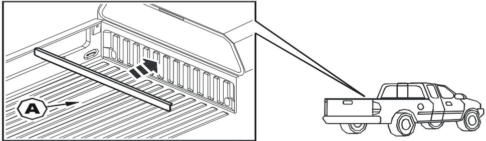
**2** Drill four evenly spaced 9/64" holes through the front bed cap (A) as shown below.
