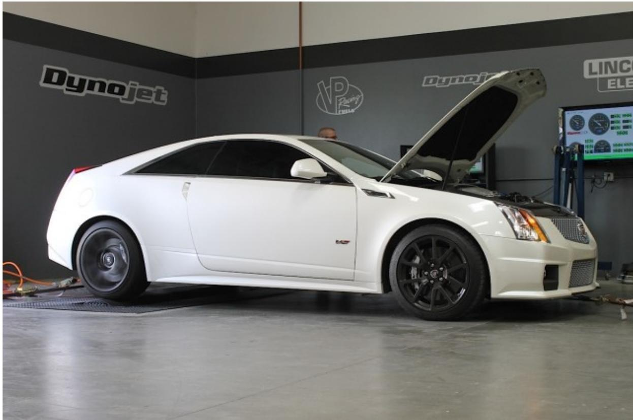
Before we got to work installing the coils, we strapped the car down on our [DynoJet 224xLC chassis dynamometer](#) to get some baseline horsepower numbers. Keep in mind that our CTS-V already has the [Lingenfelter 378 CID LSA Supercharger Upgrade](#) and a larger [Lingenfelter intercooler package](#) with dual 2-speed SPAL fans, so our starting point is going to be a lot higher than the baseline numbers for a factory car, obviously.
