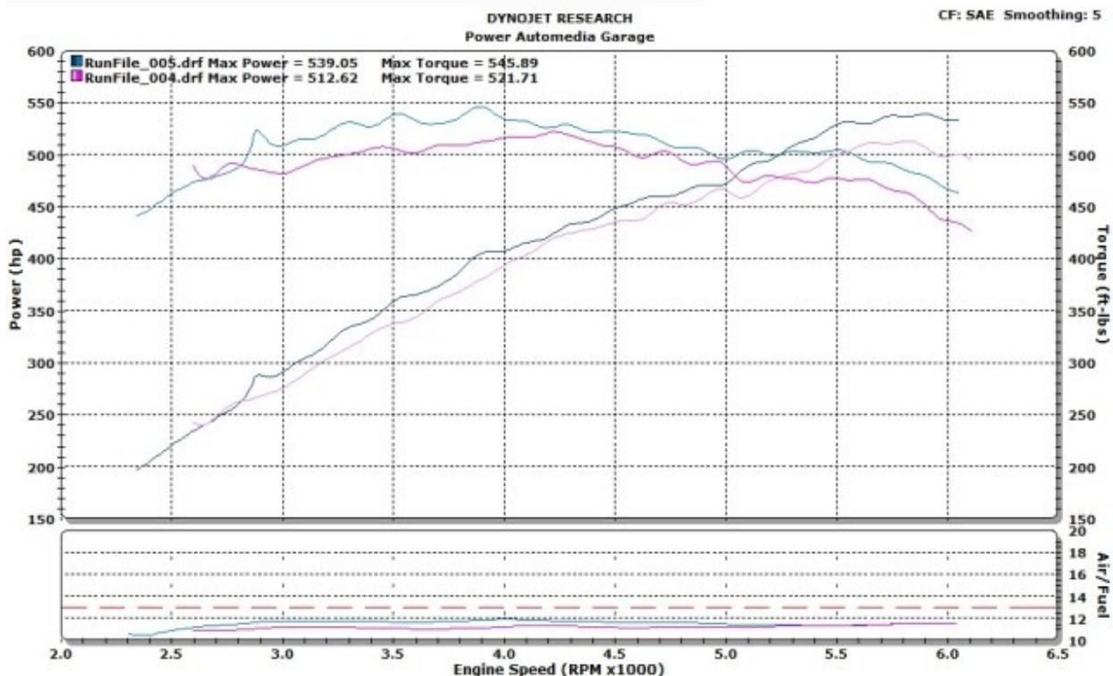
When we saw the dyno graphs after the pull we couldn't believe how much of a gain these SOS coils gave our CTS-V – a gain of **26.4 horsepower** and **24.1 pound-feet** at the wheels! That brings the CTS-V's power output up to **539 horsepower** and **545.8 pound-feet** to the ground!
