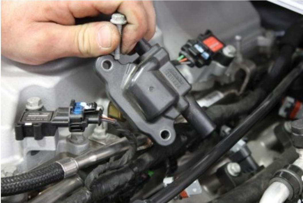
The first step of the installation is to disconnect the negative battery cable. Starting on the driver's side of the car, we removed the coil packs of all the odd-numbered cylinders, then shifted to the passenger side to remove the even-numbered coil packs, even though the install can be started from either side – we just wanted to be organized.
