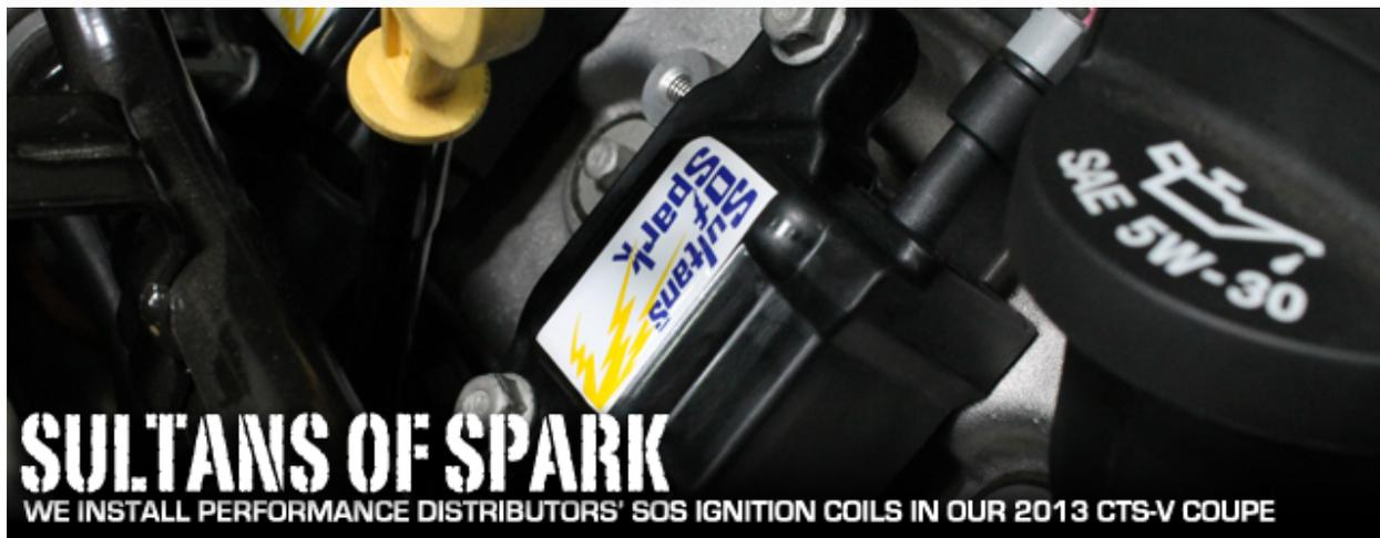
For decades, the mechanical distributor and single coil ignition system was found on just about every engine on the road, but today, distributorless ignition systems are the rule. Wasted-spark, coil-on-plug, coil-per-cylinder, or coil-near-plug are all terms you'll hear nowadays in conjunction with modern spark delivery.
