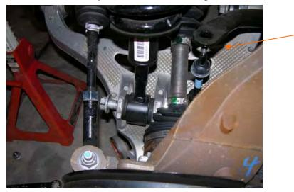
4. Disconnect the brake line from the strut tower.
