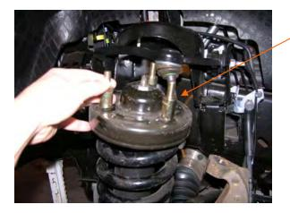
9. Install the spacer lift on top of the strut plate.
