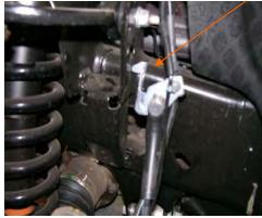
5. Separate the upper ball joint from the spindle. Use a ball joint separator or other suitable tool.
