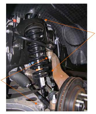
12. With the ball joint nut installed on the ball joint tighten the upper strut nuts.
