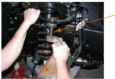
6. Remove the 3 upper strut mounting nuts on the top off the strut tower.
