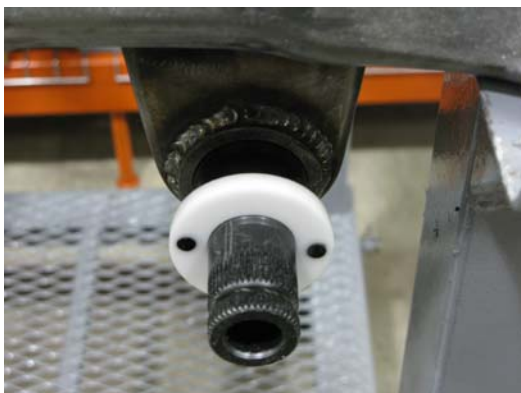
Figure 12 - Installing the Bushing & Anti-Roll Bar
