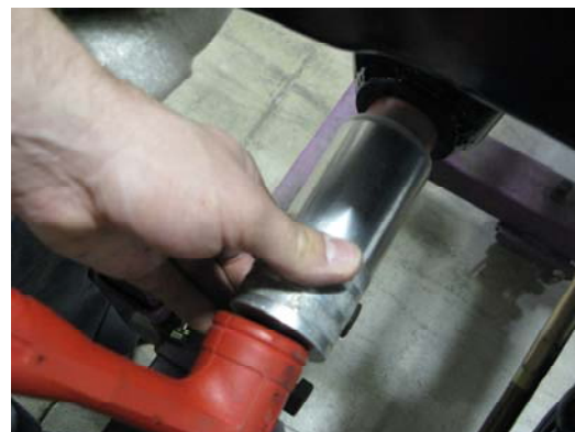
Figure 13 - Fully Installing the Bushings
