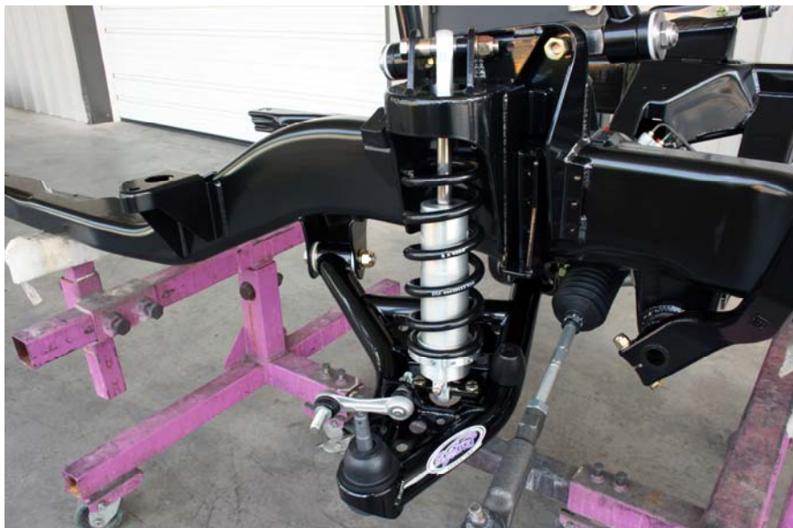
Figure 8 - Installed Coilover View (Passenger Side)
