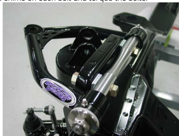
Figure 9b - Installed Upper Control Arm View
