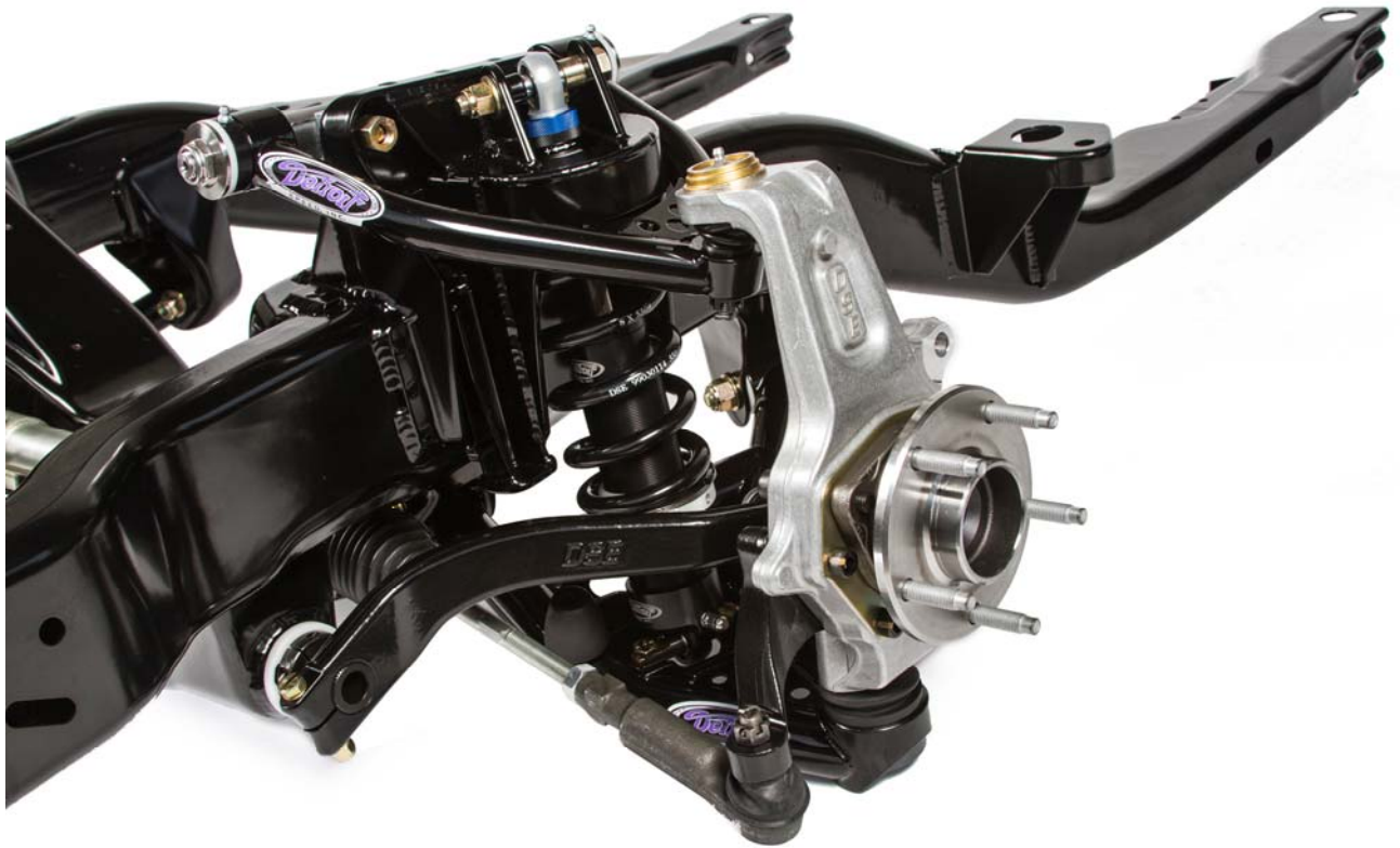
Figure 16 - Fully Assembled View (Driver Side, Front)
