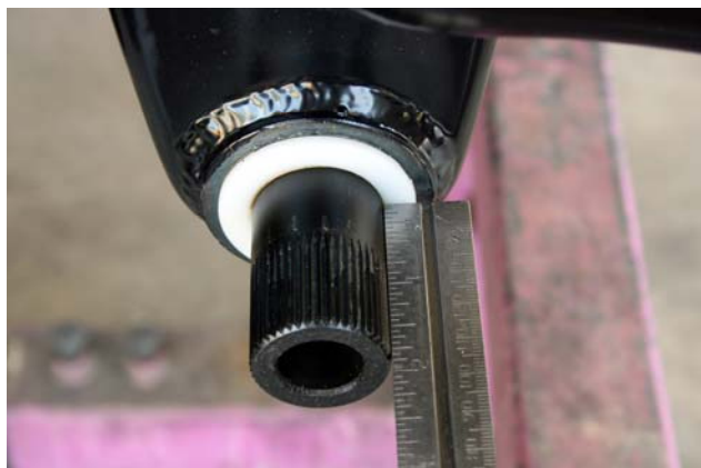
Figure 14 - Measuring the Anti-Roll Bar
