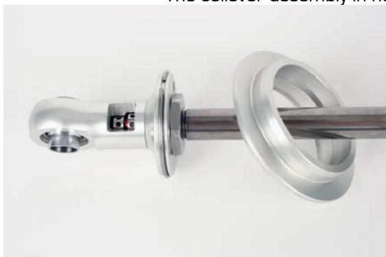
Figure 6 – Installing the Retaining Ring
