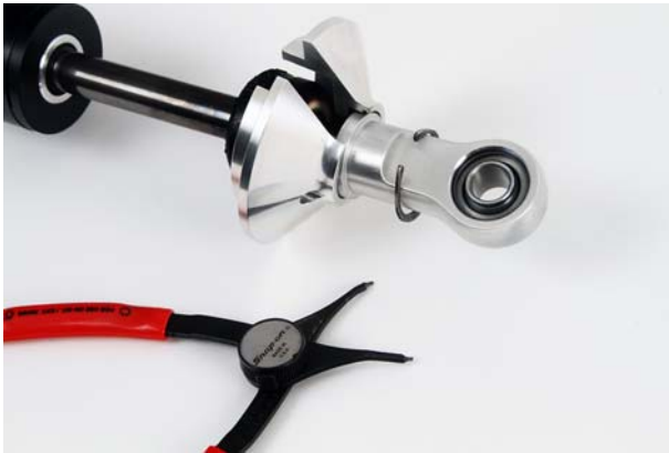
Figure 3 – Remove the Snap Ring
