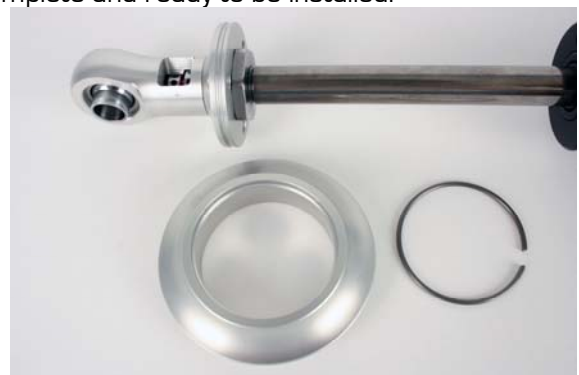
Figure 7 – Upper Spring Seat & Retaining Ring
