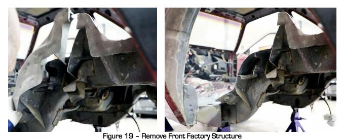
24. Cut through the rear side of the upper shock mount and around the factory wheel tub flange to remove this section of structure from the vehicle (Figure 20).
