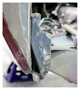
Figure 30 - Remove Inner Wheel Tub Layer
