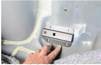
Figure 43 - Seat Belt Relocation Bracket
