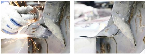
Figure 28 - Remove Seat Belt Anchor
