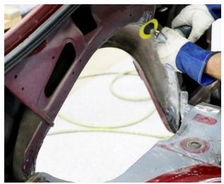
Figure 32 - Grind Sheet Metal
