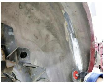
Figure 8 - Remove Undercoating
