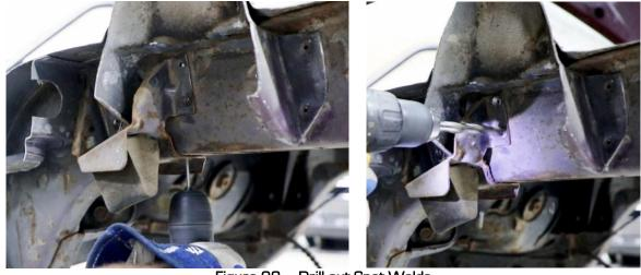
Figure 23 - Drill out Spot Welds
