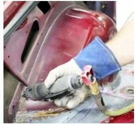
Figure 17 - Cutout Inner Wheel Tub
