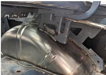
Figure 49 - Re-attach Trunk Hinge Bracket
