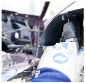
Figure 26 - Remove Spring Perch Spot Welds
