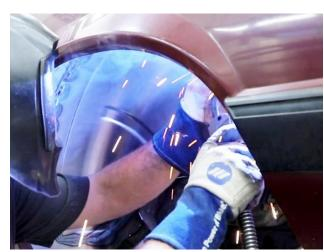
Figure 40 - Finish Weld around Mini-Tub
