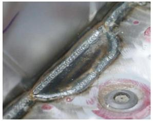
Figure 42 - Weld Closeout
