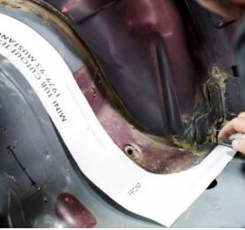
Figure 15 - Locate Front Template
