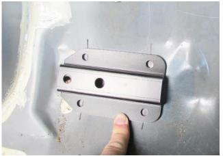
Figure 45 - Transfer Punch Holes
