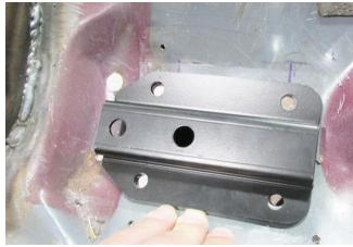
Figure 46 - Drill Bracket Mounting Holes
