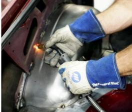
Figure 38 - Tack Weld Mini-Tub
