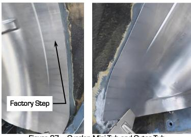
Figure 37 - Overlap Mini-Tub and Outer Tub
