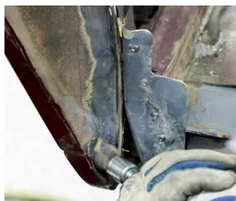
Figure 31 - Adjust Flange
