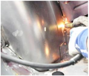
Figure 39 - Tack Weld Flange
