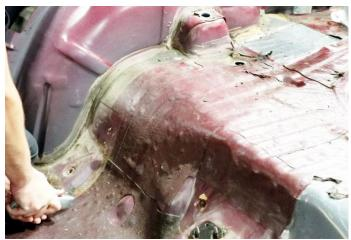
Figure 4 - Remove Trunk Pan Material
