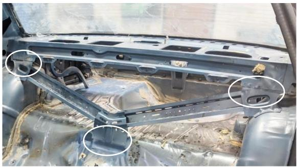
Figure 3 - Remove Wheel Tub Brackets
