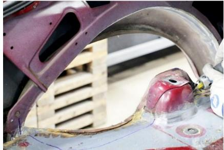
Figure 18 - Cut on Template Line
