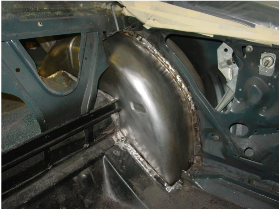
Figure 12 - Welded Tub View (Passenger Compartment)
