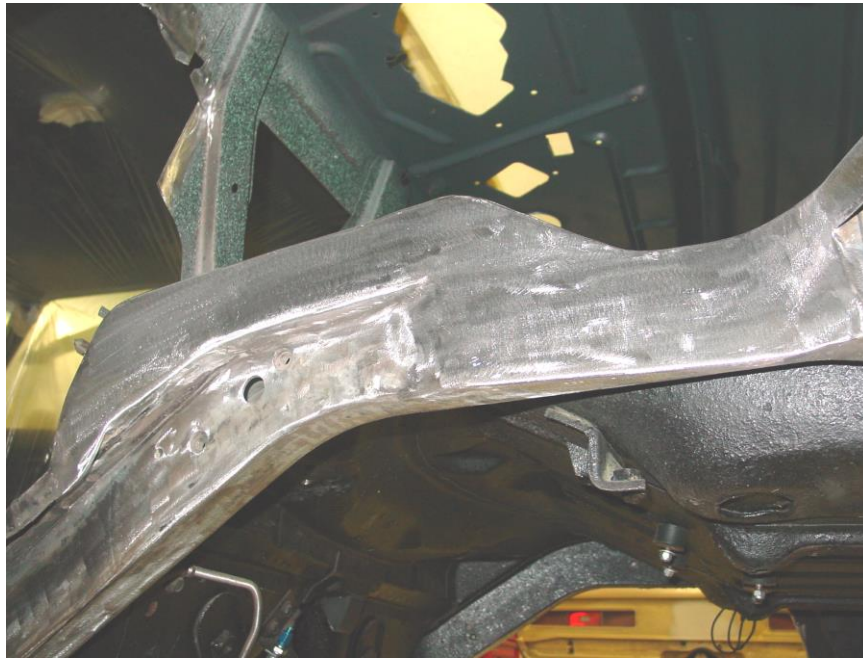
Figure 7 - Framerrail with Closeouts Installed
