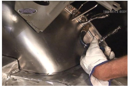
Figure 38 – Clamp and Weld to the Vehicle
