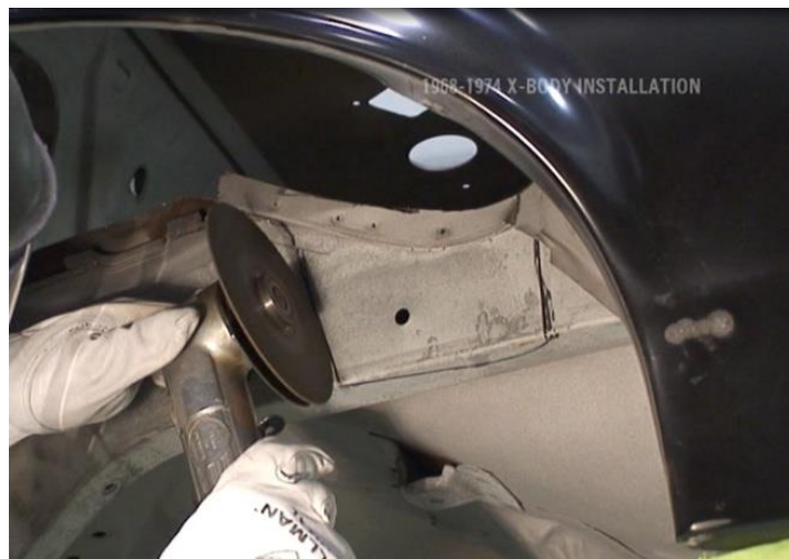
Figure 18 - Notch the Framerail
