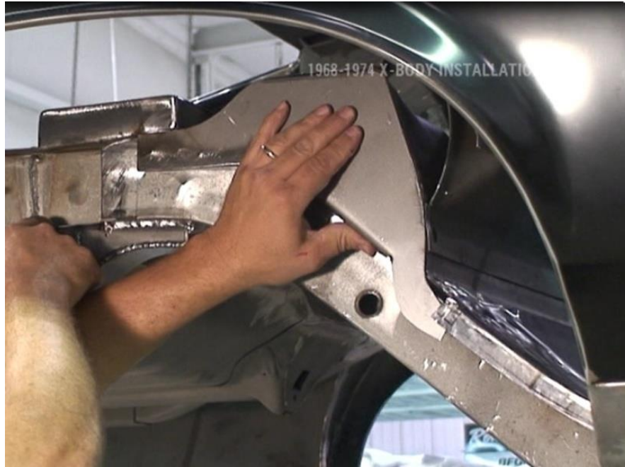
Figure 36 - Passenger Side Closeout
