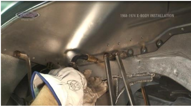
Figure 38 – Clamp and Weld to the Vehicle
