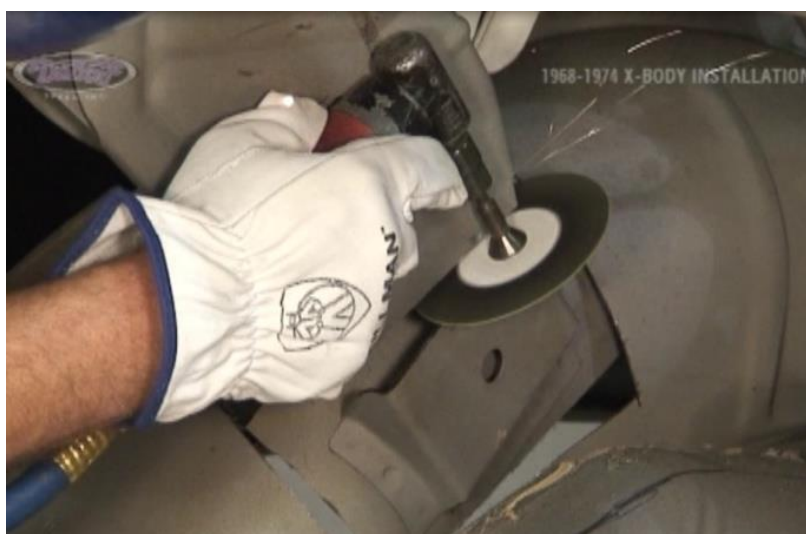
Figure 12 - Cut and Remove the Hinge Mount
