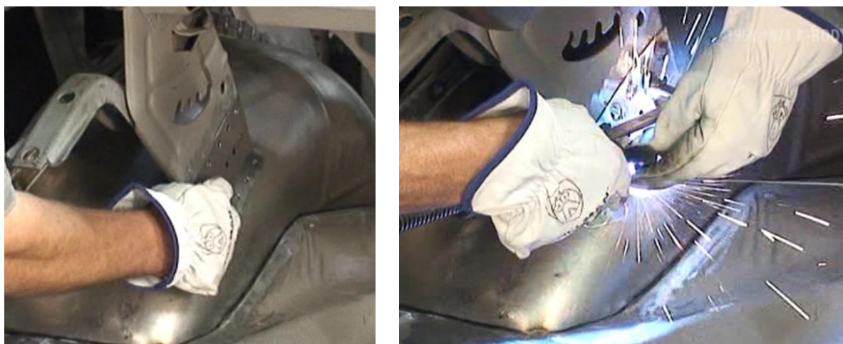
Figure 32 – Fabricate and Weld the Decklid Support
