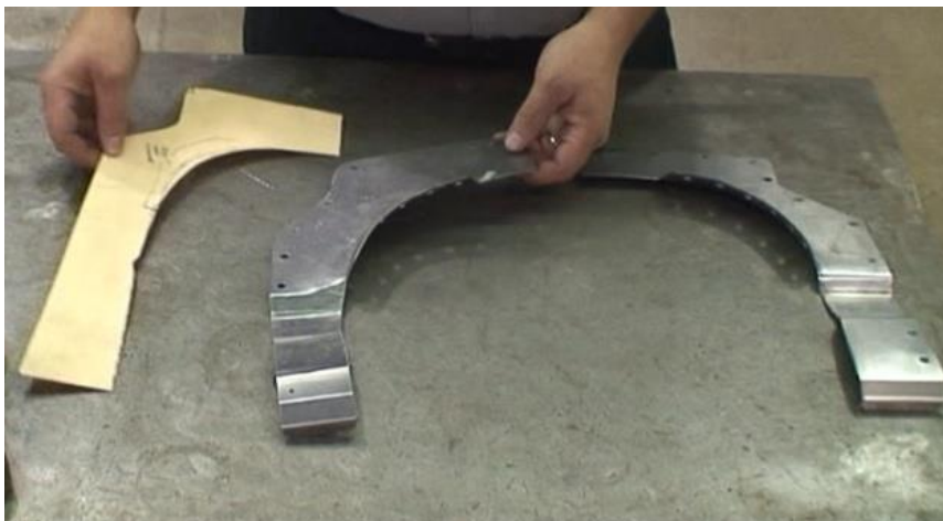
Figure 41 – Seat Back Brace
