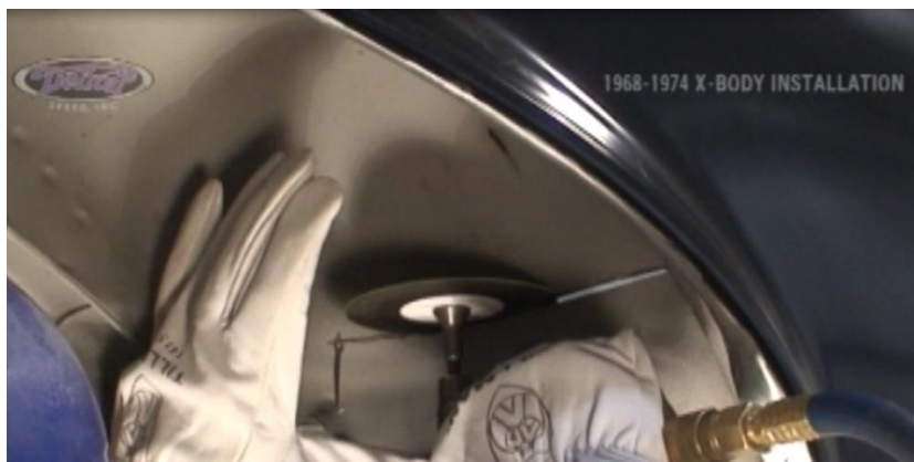
Figure 10 – Start Cutting the Stock Tub
