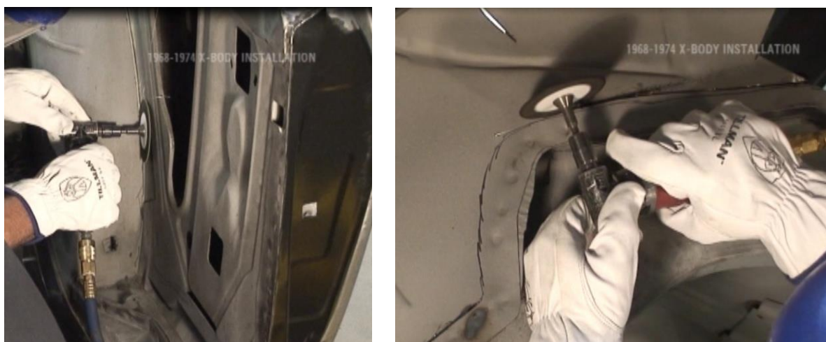
Figure 13 - Cut Pre-Marked Lines
