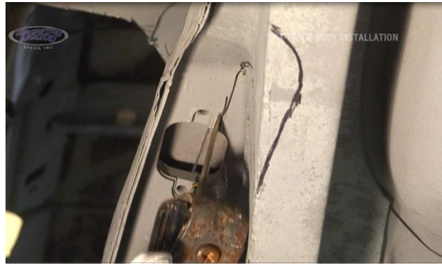
Figure 17 - Cutting along the Framerail
