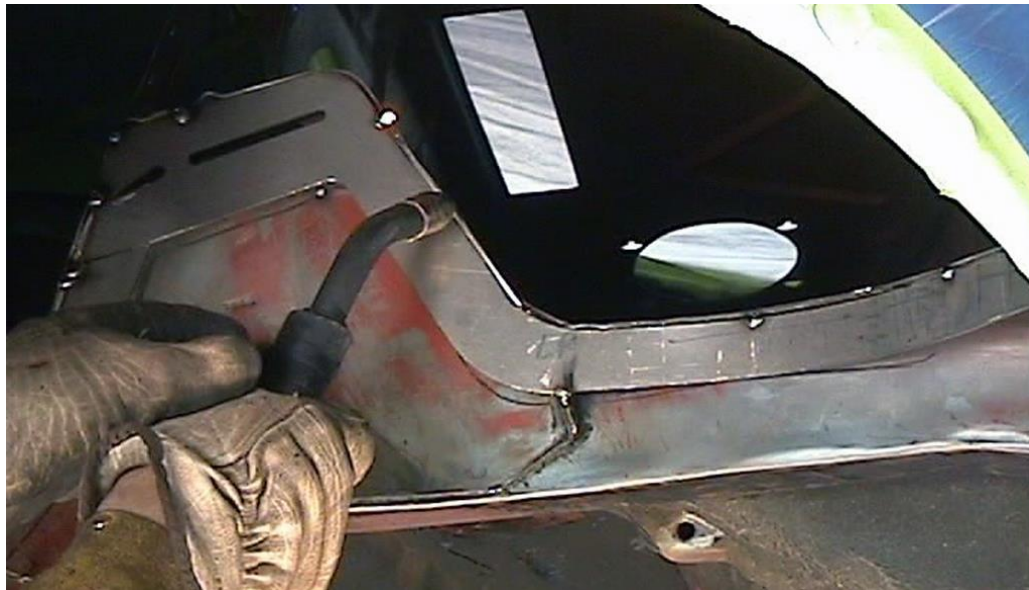
Figure 14 - Tack Weld Tub Flanges
