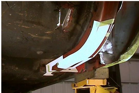
Figure 3 - Inboard Frame Rail Template
