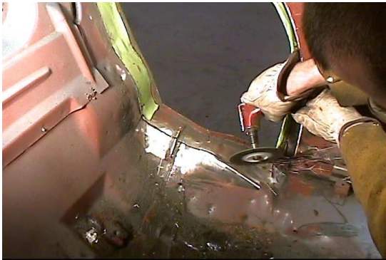
Figures 8 and 9 - Metal Removal for Clearance of Detroit Speed Mini Tubs
