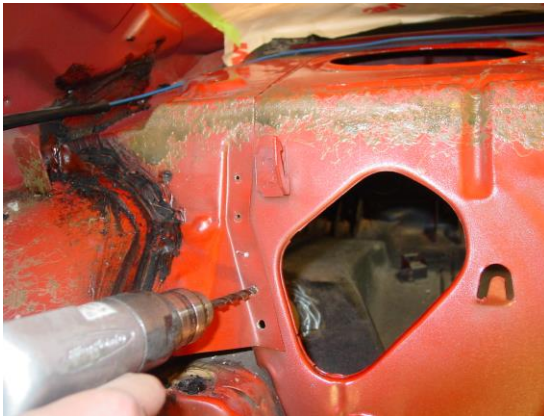
Figure 1 - Seat Support Cut Line
