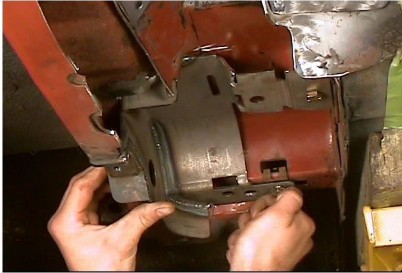
Figure 8 - Leaf Spring Pocket Mount
