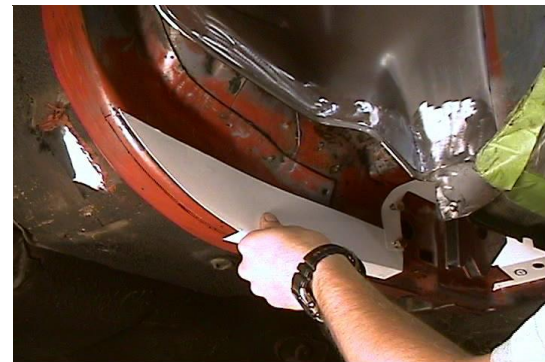
Figure 4 - Outboard Frame Rail Template
