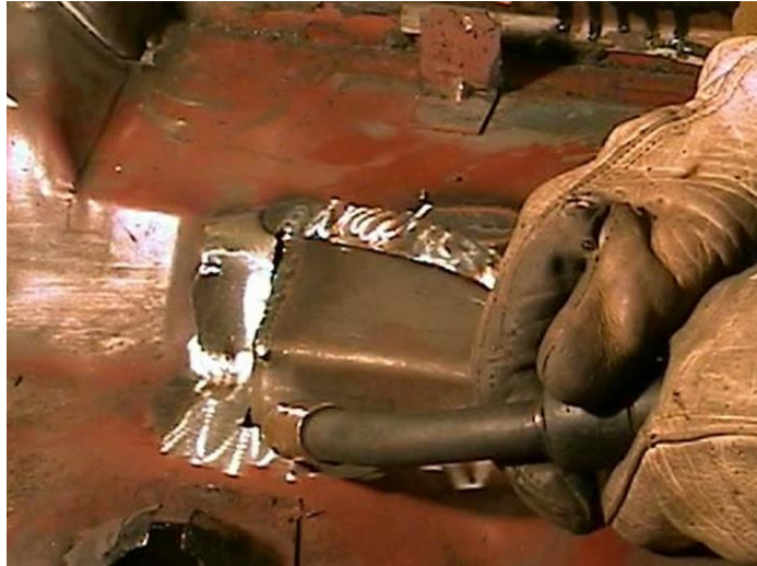
Figure 10 - Welding the Leaf Spring Pocket
