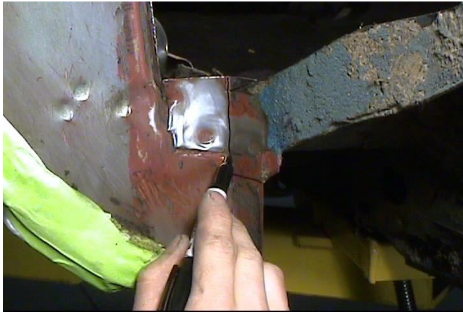
Figure 7 - Marking Tab for Removal
