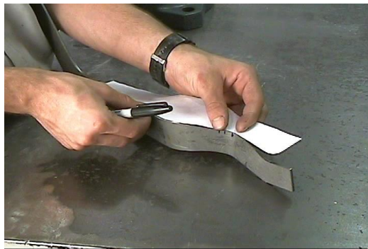
Figure 11 - Front Template Bend Profile
