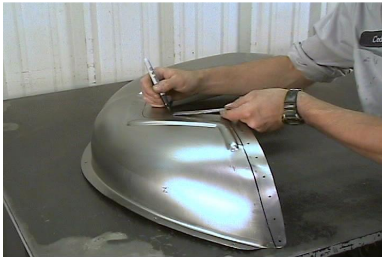
Figure 16 - Mark Tub Mounting Surfaces
