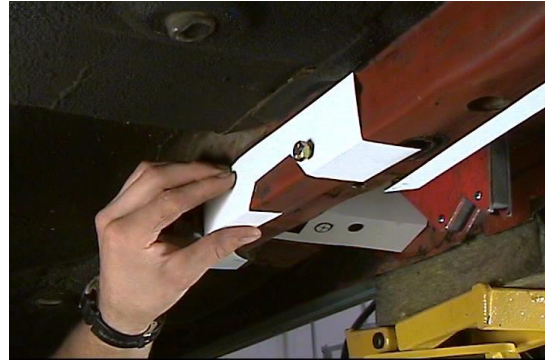
Figure 2 - Leaf Spring Pocket Template - B
