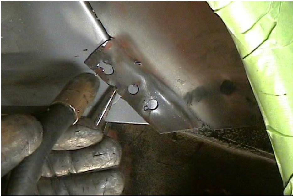
Figure 20 - Wheel Tub Overlap
