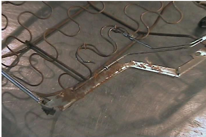
Figure 1 - Rear Seat Frame Modification
