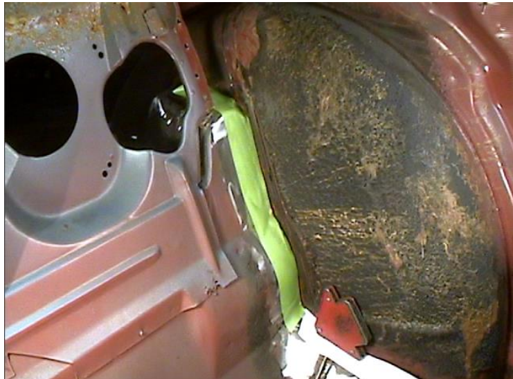
Figure 6 - Cut Line Extension Using 2" Tape
