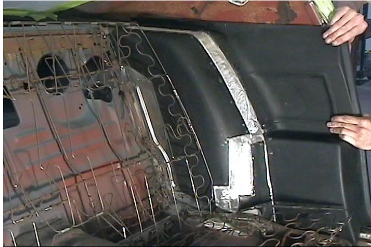
Figure 3 - Modified Interior Quarter Trim Panels
