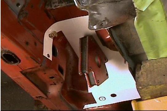
Figure 1 - Leaf Spring Pocket Template - A
