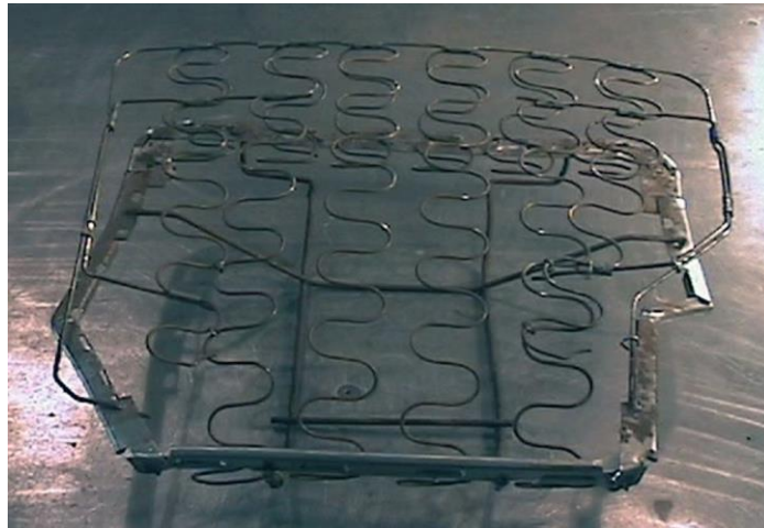
Figure 2 - Narrowed Rear Seat Frame
