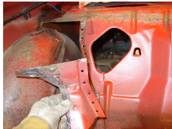
Figure 2 - Seat Support Removed
