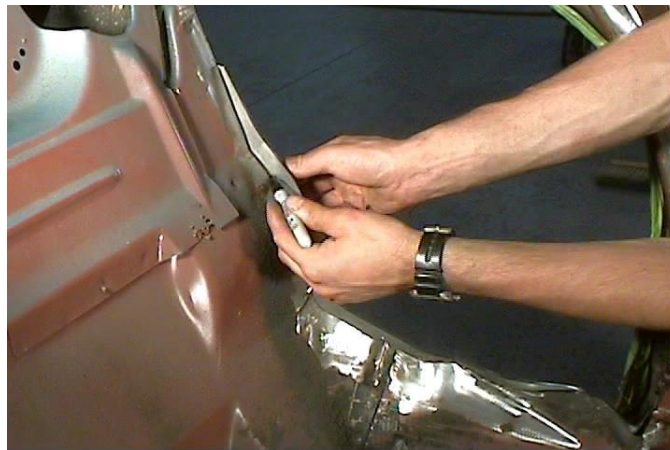
Figure 13 - Marking Front Template to Floor Pan Profile
