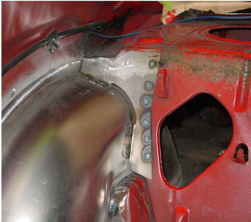
Figure 22 - Seat Back Bracket Installed
