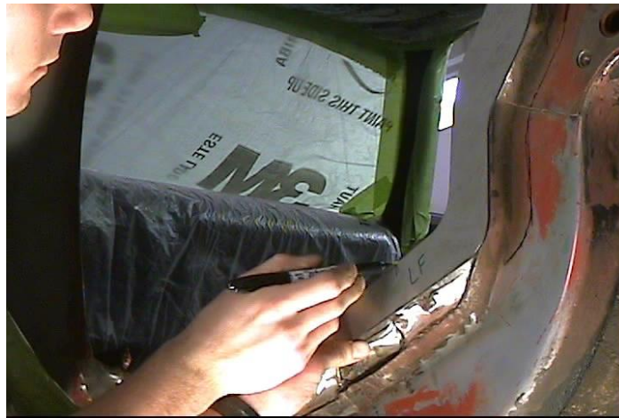
Figure 10 - Front Flange Alignment
