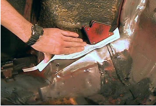
Figure 4 - Inner Wheelwell Front Template
