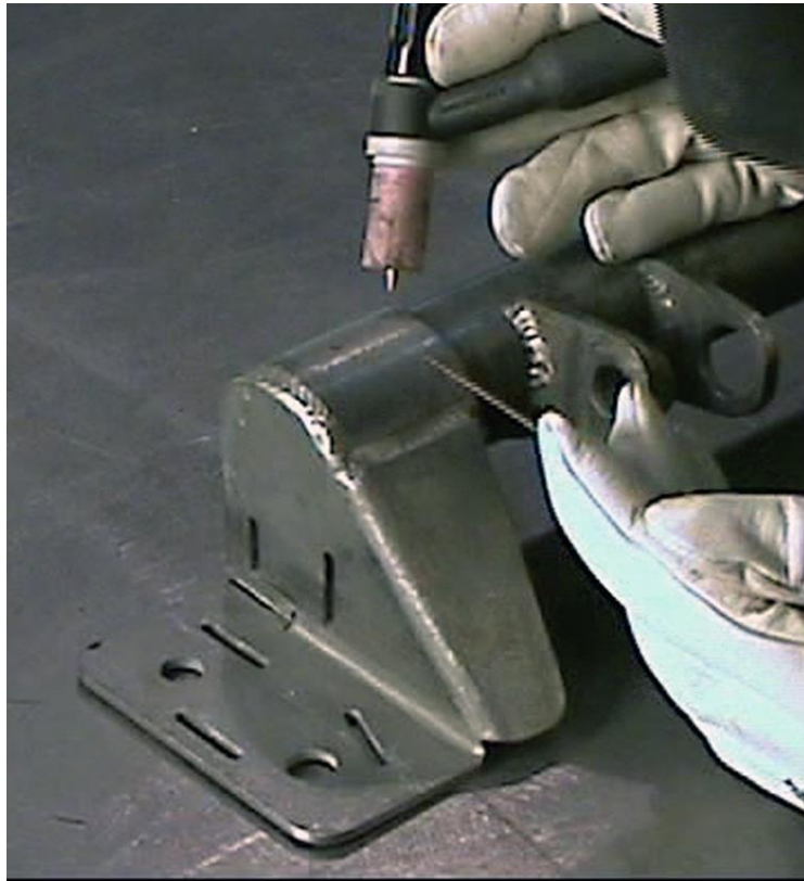
Figure 1 - Weld End Caps to Crossmember
