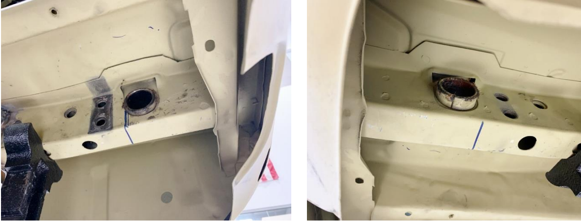
Figure 1 - Remove Shackles & Bushings
