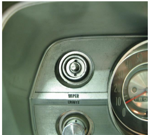
Figure 7 - Wiper Switch Bezel
