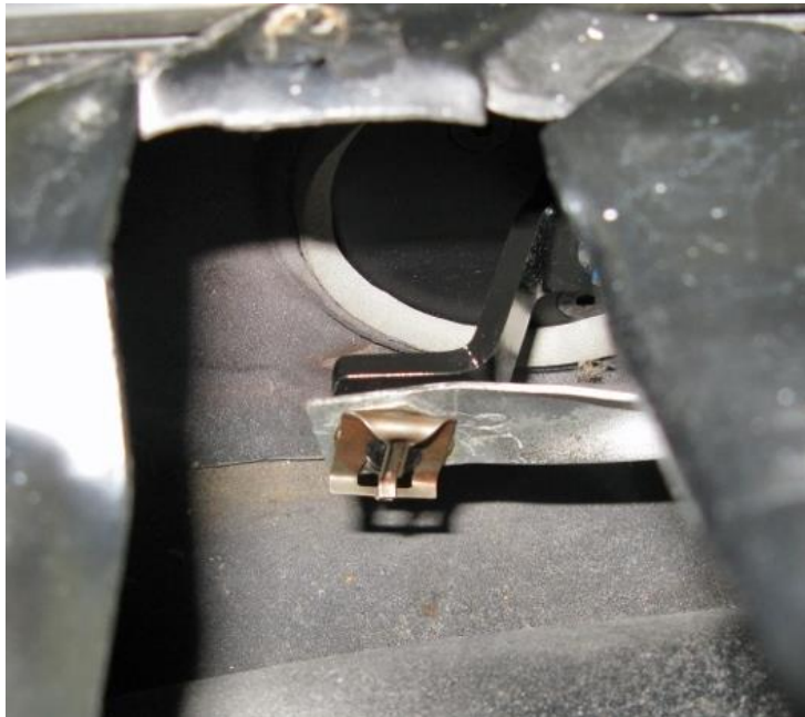
Figure 4 - Attach Pitman Arm to Wiper Linkage
