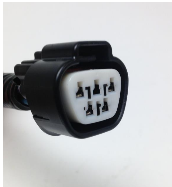
Figure 10 - Wiper Motor Connector
