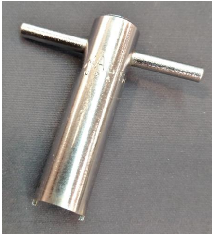
Figure 5 - Wiper Switch Removal Tool
