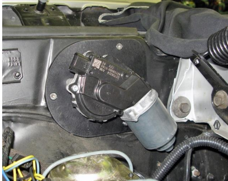
Figure 3 - "Box" Style Wiper Motor
