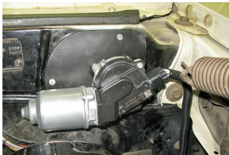
Figure 2 - "Can" Style Wiper Motor
