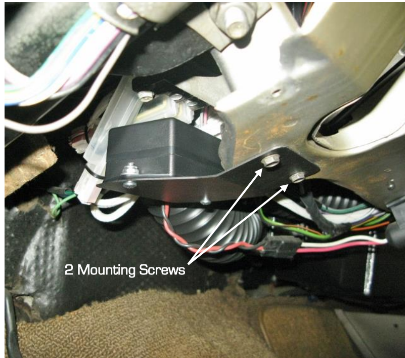
Figure 15 - Install Module & Mounting Plate
