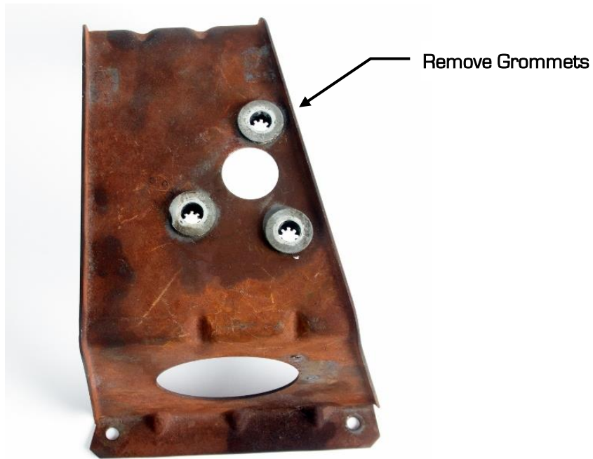
Figure 2 - Factory Wiper Motor Mounting Bracket
