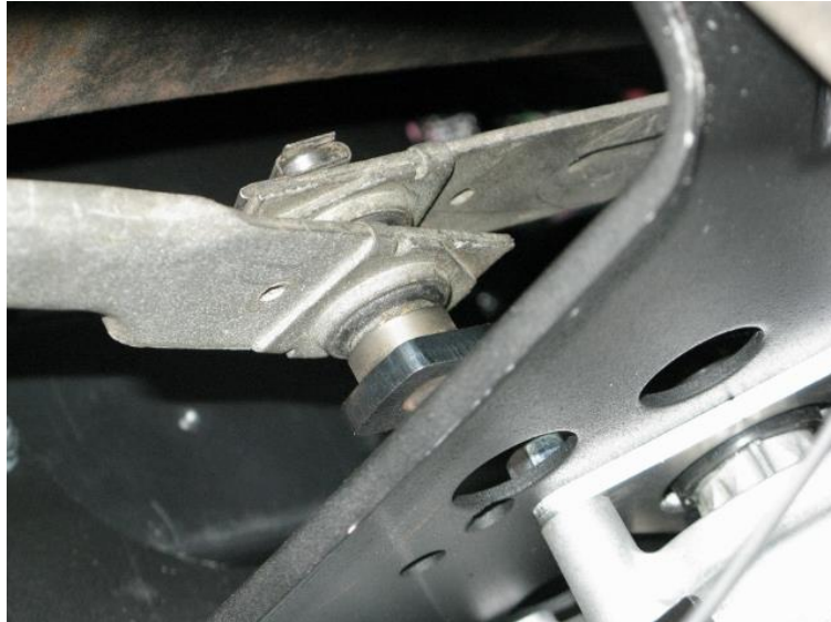
Figure 6 - Attach Wiper Linkage to Pitman Arm
