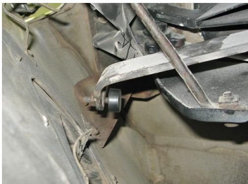
Figure 10 – Install Round Bumper
