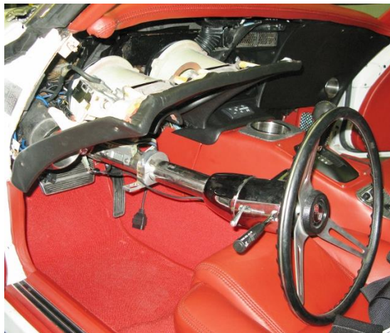
Figure 22 - Remove Dash Pad
