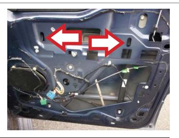
**STEP 5:** Manually slide the window glass to align the screws attaching the window glass to the window regulator.
