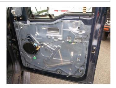
STEP 7: Connect the interior door handle cable to the interior door handle.
