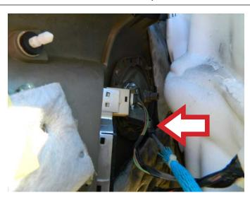
**STEP 9:** Connect the power door lock switch.
