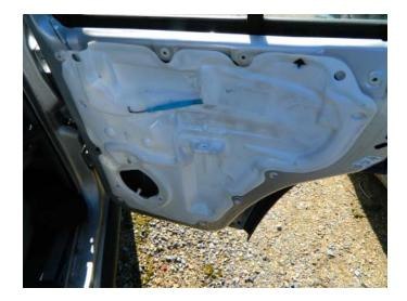
**STEP 9:** Operate the power window switch and lower the window glass to expose the two (2) window glass mounting bolts.
