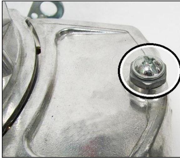
Use a wrench to hold the nut while turning the screw with a Phillips head screwdriver Figure 11
