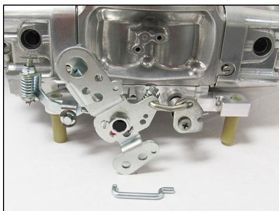
Speed/Road Demon™ mechanical secondary carburetors are supplied with the progressive link.
