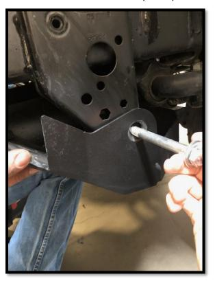
10. Once the two lower skid plate bolts are loosely installed, rotate skid plate up, and use the provided bolts to secure the top portion of the skid plate to the main bumper and wing. Once installed, you can secure the lower frame horn bolts.
