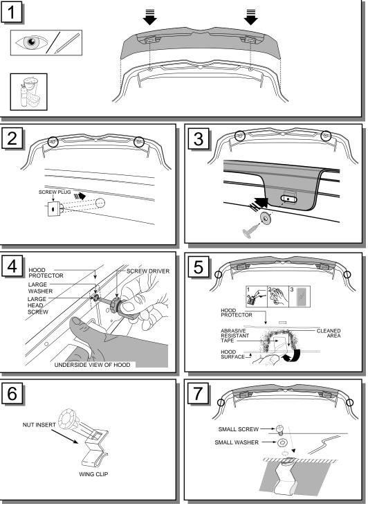
4 • While maintaining thumb pressure against the underside of the Hood Protector, insert large washer and self-tapping screw into the screw plug and tighten screws. Do not fully tighten yet. Ensure the Hood Protector is centralised on hood then fully tighten screws. DO NOT OVERTIGHTEN SCREWS.
