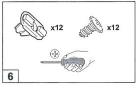
Ensure that all of the correct hardware is in the hardware kit. (screwdriver not supplied)
