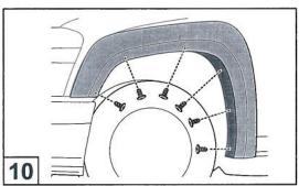
Install the supplied screws through the Fender Flare into the previously installed screw plugs.
