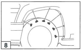
Install the supplied screw plugs into the existing slots as shown.
