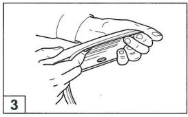
Remove approximately 2" (50mm) of the protective liner from the extrusion. Fit the extrusion to the Fender Flare along the edge that comes in contact with the vehicle's body panel.
