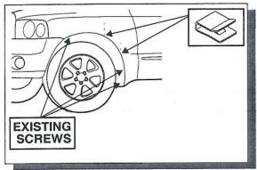
5. Note the correct hardware and existing screws position as shown. Also note the clips position.
