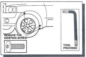
**6** Remove the existing screws on vehicle as previously noted, using the tool provided.
