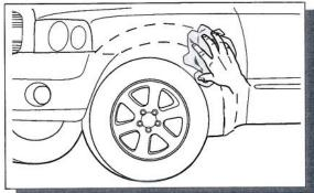
• Wash the areas of contact on the vehicle and wipe dry both the vehicle and the Fender Flare with a clean cloth. Ensure inside of Fender Flare where extrusion is attached is clean.
