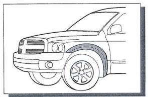
7. Fit the Fender Flare and align it with the existing screw positions. Secure the Fender Flare to vehicle by replacing the existing screws.
