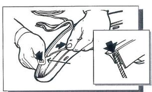
3 Pulling at right angles from the extrusion remove the liner from the extrusion in small portions and apply thumb pressure to ensure that it adheres to the Fender Flare.
