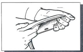
2. Remove approximately 50mm (2") of the protective liner from the extrusion. Fit the extrusion to the Fender Flare along the edge that comes in contact with the vehicles body panel.
