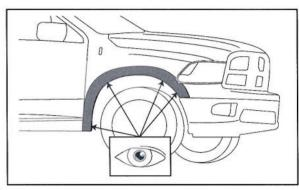
9. Place the Fender Flare on the vehicle into the position of best fit. Note where the slots in Fender Flare at positions A,B,C and D align with the existing screws in the vehicle. Remove Fender Flare.
