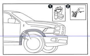
**3.** Wash the areas of contact on the vehicle and wipe dry both the vehicle and the Fender Flares with a clean cloth. Ensure inside of Fender Flares where extrusion is attached is clean, using the alcohol wipes provided and wipe away any residue with a dry, clean cloth.
