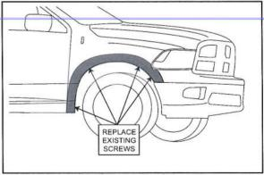
11. Replace the Fender Flare on the vehicle into position of best fit. Complete installation by replacing the previously removed screws at position A, B, C and D, ensuring the Fender Flare is located firmly and extrusion is neat against the vehicle fender.
