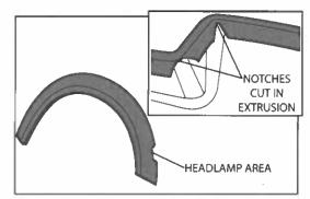
**6.** Cut notches in extrusion tape to allow it to fit neatly around headlamp area of flare as shown.
