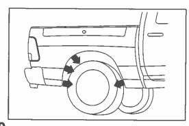
**9.** Remove the previously noted existing screws and retain for re-installation.
