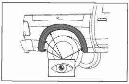
Place the Fender Flare on the vehicle into the position of best fit. Note where the slots in Fender Flare at positions A,D,E and F align with the existing screws in the vehicle. Remove Fender Flare.
