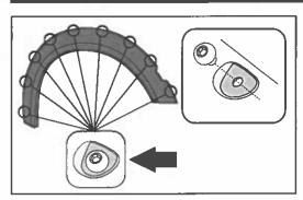
Attach 9 extruded plastic bolts. Begin by peeling back the white tape liner from the bottom side of the extruded plastic bolt and press until it snaps into place.
