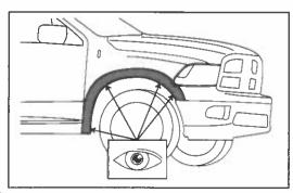
**9.** Place the Fender Flare on the vehicle into the position of best fit. Note where the slots in Fender Flare at positions A,B,C and D align with the existing screws in the vehicle. Remove Fender Flare.
