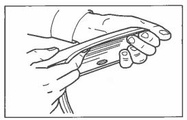
4. Remove approximately 2" (50mm) of the protective liner from the extrusion. Fit the extrusion to the Fender Flare along the edge that comes in contact with the vehicle's body panel.
