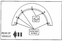
7. Note the correct hardware for positions A, B, C, D, E & F (Right Fender Flare shown).
