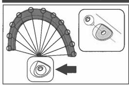
Attach 11 extruded plastic bolts. Begin by peeling back the tape liner from the bottom side of the extruded plastic bolt and press until it snaps into place.
