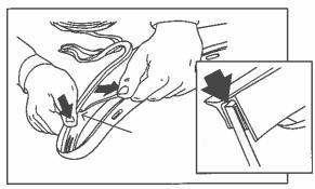
**5.** Pulling at right angles to the extrusion, remove the liner from the extrusion in small portions and apply thumb pressure to ensure that it adheres to the Fender Flares.
