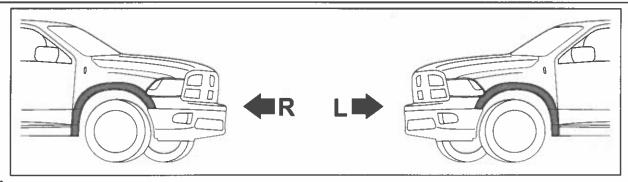
1. Ensure that both left and right hand Fender Flares suit the profile of the vehicle. Note the areas where the Fender Flares come in contact with the vehicle. NOTE: Before fitting Fender Flares remove any mouldings, strips or existing flares from the wheel arch. If there is a body side moulding, mark where the moulding is to be cut, alternatively the Fender Flares can be cut to go around the moulding. Be sure to allow enough room for the extrusion.
