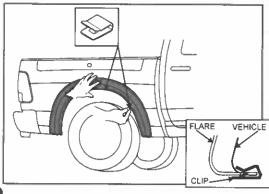
10. Replace Fender Flare on the vehicle into position of best fit. Take the supplied snap clips and fix them into positions B and C, as shown, ensuring the notch in clip locates securely into the slot in the Fender Flare.
