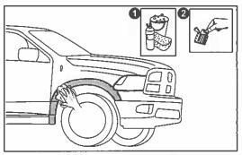
Wash the areas of contact on the vehicle and wipe dry both the vehicle and the Fender Flares with a clean cloth. Ensure inside of Fender Flares where extrusion is attached is clean, using the alcohol wipes provided and wipe away any residue with a dry, clean cloth.
