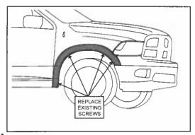
11. Replace the Fender Flare on the vehicle into position of best fit. Complete installation by replacing the previously removed screws at position A, B, C and D, ensuring the Fender Flare is located firmly and extrusion is neat against the vehicle fender. Repeat process for the other side of the vehicle.
