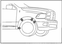
$10\overline{.}$  Remove the previously noted existing screws and retain for re-installation.
