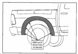
11. Complete installation by replacing the previously removed screws at position A, D, E and F, ensuring the Fender Flare is located firmly and extrusion is neat against the vehicle fender.
