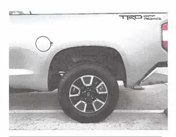
**STEP 5:** Clean the body area where the Fender Flares will make contact. Ensure fenders are dry prior to install.
