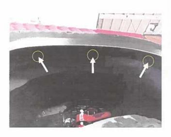
**STEP 10:** Locate the (3) remaining mounting slots on the Fender Flare as shown.
