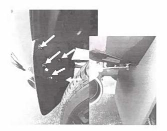
**STEP 4:** Using a 10mm socket / wrench remove the 5 screws from the inner area of the mud guard. Using a small flat screwdriver disengage the pin from the plug at the base of the mud guard. Remove mud guards completely and retain all components. Mud Guards cannot be installed with these Fender Flares.
