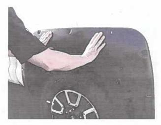
STEP 6: Hold Fender Flare on the vehicle in the position of best fit. Note where all the slots in the Fender Flare align with existing mounting holes in the vehicle.
