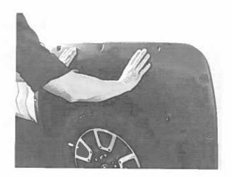
STEP 9: Working from top to bottom at these same (3) slot positions, hold and align the spacers with the slots and use the Long Screws to go through the spacers and into the corresponding factory holes.
