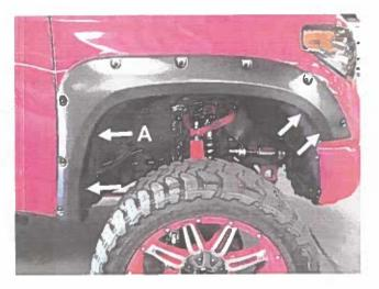
**STEP 6:** Hold Fender Flare on the vehicle in the position of best fit. Note where above marked slots in the Fender Flare, align with the existing screws / mounting holes in the vehicle. Make special note of "A" Remove the Fender Flare.
