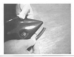
STEP 2: Attach the included rubber seal to the Fender Flares along the top leading edge where the Flare will make contact with the exterior painted vehicle body. Peel back 2" of the adhesive liner and apply the double sided tape to the inside surface of the Fender Flare, peeling back a few inches at a time and applying pressure to secure rubber seal to Fender Flare.
