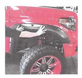
**STEP 12:** If necessary, make minor adjustments to the flare's position to achieve the best fit. Ensure rubber seal is sitting flat against vehicle. When satisfied fully tighten all screw locations, in the above order in which they were just installed.
