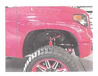
STEP 5: Clean the body areas where the Fender Flares will make contact. Ensure fenders are dry prior to install. Turn tires facing outward to provide additional room and ease hardware installation per side.
