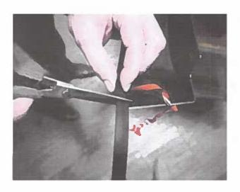
**STEP 3:** Trim rubber seal at end of Fender Flare. Save extra rubber seal for install on opposite side Fender Flare and discard any excess once both sides are complete.
