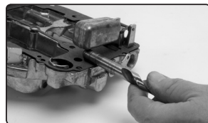
Checking float level with a 7/16" drill bit
