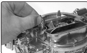
Metering rods can be changed without removing the lid from the carburetor
