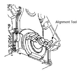
Figure 2 - Front Cover Alignment Tool
