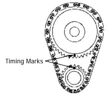
Figure 1 - Timing Mark Alignment
