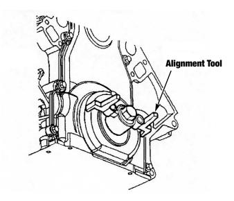
Figure 2 - Front Cover Alignment Tool
