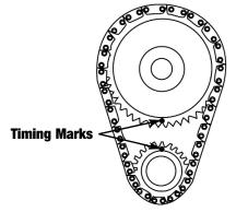
Figure 1 - Timing Mark Alignment
