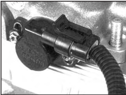
The Throttle Position sensor attaches to the harness with Connector J5.
