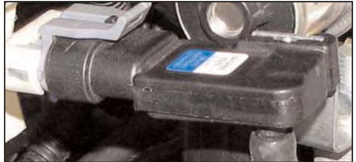
The Manifold Absolute Pressure sensor attaches to the harness with Connector J17.
