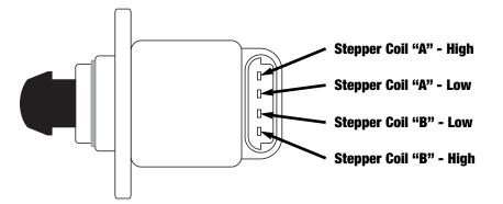
Figure 2 - Hitachi Linear IAC Motor (Pulse Width Modulated)
