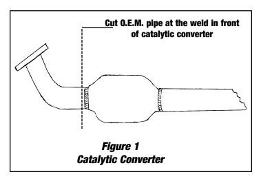
**NOTE:** Make sure to have the correct pipe on each side of the catalytic assembly or it will not set right. I.D. number is stamped on each part: 25-9670 - Left, 25-9671 - Right.
