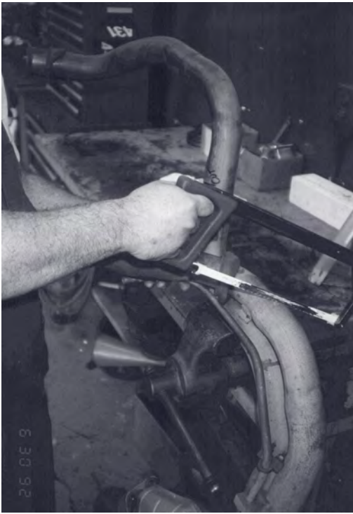
Figure 4a After marking pipe to be cut, clamp securely, then cut with hacksaw
