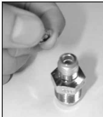
Shown above is the new burst disc being installed on the Racer Safety Blow Off Adapter. Be sure when installing the burst disc that you do not collapse the sides of the disc or damage the disc in any way.
