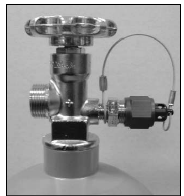
Installed on this valve is the Racer Safety Blow Off Adapter and Diffuser Cap. Whenever the bottle is not installed in the vehicle, be sure the Diffuser Cap is installed on the PRD. Also, be sure never to overtighten the Diffuser Cap or Blow Down Tube on the PRD.
