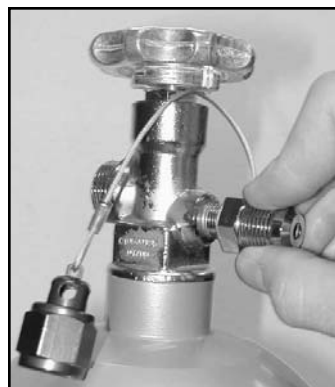
Be sure to place the wire rope loop on the PRD. Hand-tighten the PRD into place as shown above paying special attention to making sure the Burst Disc remains in place. Once hand-tight, torque to 17 ft. lbs. using a properly calibrated torque wrench.
