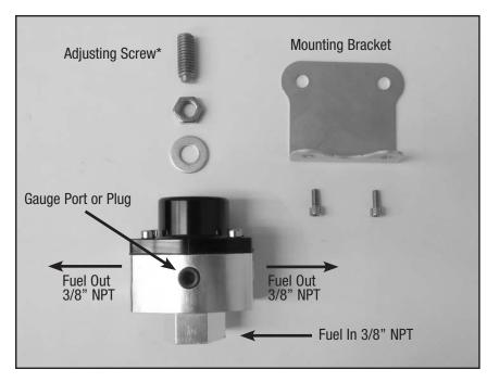
**\*NOTE:** Thread adjusting screw down (clockwise) to increase fuel pressure; thread adjusting screw up (counter-clockwise) to decrease fuel pressure.
