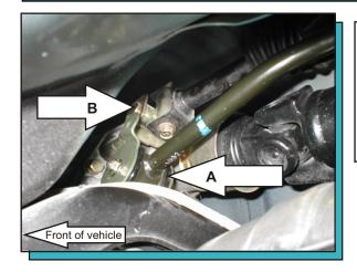
**Note:** Do not remove the upper shifter linkage (See arrow B). Remove old rubber bushing from the lower shifter linkage at the transmission mounting stud. (See arrow A) Install the new poly bushing into the linkage with the part number (1170) facing outward away from transmission.
