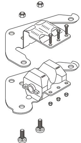
NOTE: The 3/8" bolts have a square on them which will "bite" on the inside of the 1/2" hole and keep them from turning. However, it may be necessary to use locking pliers to keep the bolt from turning while applying the proper torque.
