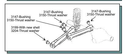
The thrust washers are designed to prevent the control arm from walking side-to-side by accepting side load pressure created during hard cornering. Most kits contain more than one part #. It is very important to install them at the correct location.
