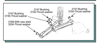
The thrust washers are designed to prevent the control arm from walking side-to-side by accepting side load pressure created during hard cornering. Most kits contain more than one part #. It is very important to install them at the correct location. **See illustration**
