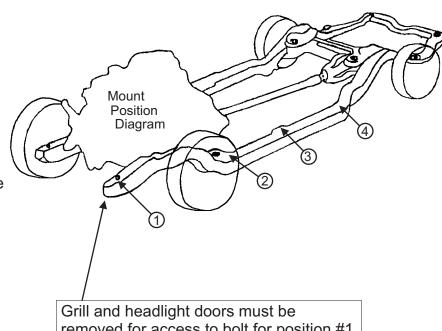
removed for access to bolt for position #1
