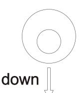
Bushings must be installed with offset hole down and centered in the 6 o'clock position.
