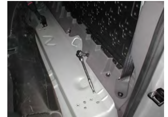
Remove rear panel bolts.
