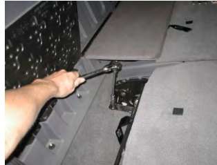
Remove rear seat bolts.
