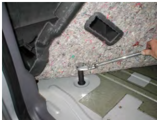
Lift carpet in rear of cab.
