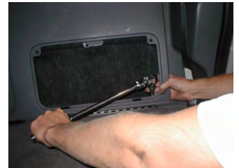
Flex out panel to access bolt.
