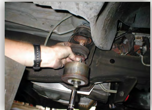
Remove body mounts
