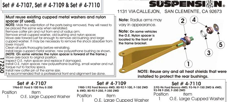
2 7049 bushing 2 7002 bushing 3 O.E. Nylon Spacer 3 Not Used 4 7004 bushing 7049 bushing 4 O.E. Small Washer 5 5 O.E. Small
