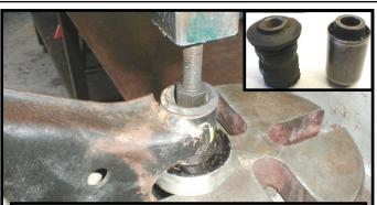
Nissan used 2 different bushings in the front position. One has a outer metal shell and must be pressed out. The other does not have an outer metal shell and can be pushed out with an arbor press. The I.D. of the O.E. control arm is Ø1.265" and is the same size for both.
