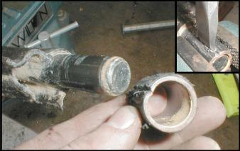
The sleeve will need to come off the rear pin. It's a tight press fit. With a hammer and chisel, make a groove along its length, this will relieve the press fit. The sleeve will then slide off by hand.
