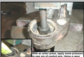
with an arbor press, apply some pressure to rear pin of control arm. Using a razor knife, cut the rubber bushing to separate the 2 parts.
