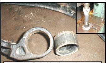
Outer metal shell of O.E. bushing must be removed. I.D. of casting for rear bushing is Ø1.930". After pressing out OE bushing, remove all sharp edges from casting.
