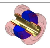
Apply grease to all metal parts that contact the polyurethane bushings.
