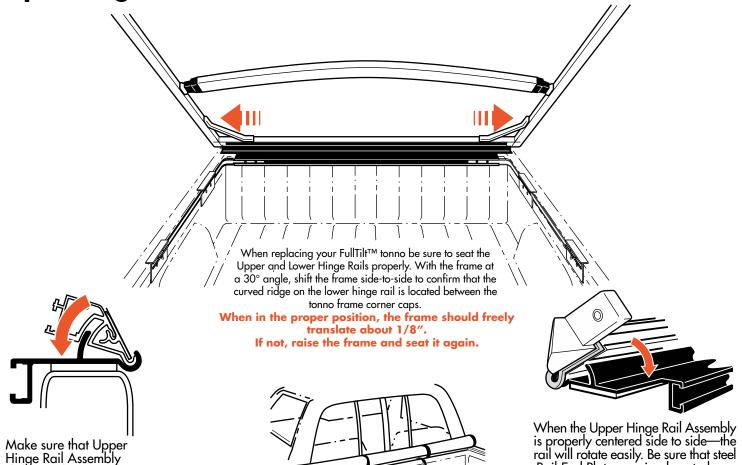
If you need to tow your vehicle backward, be sure to release the cover and stow against the hinge rail using Velcro® straps provided.
