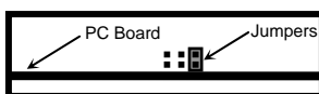
Setting 3 – Most responsive (For trucks without injectors or if smoke is not a concern)
