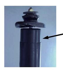
You must remove the rear shock, then, remove the upper mount to access the rear bump stop which is located underneath the OE dust boot
