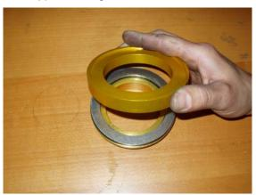
3. Disassemble the upper half of the upper bearing as shown above.
