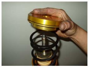
5. Install the upper bearing assembly back onto the pro street coilovers as shown above.
