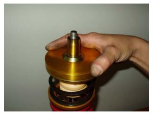
6. Install the provided spacer on top of the bearing plate as shown above.
