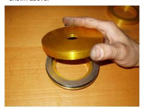
4. Now install the new upper bearing plate onto the lower half from step 3 as shown above.
