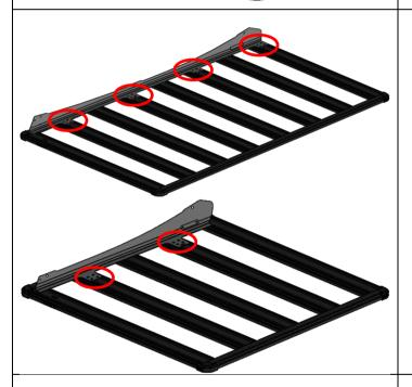
7. Check the position of the mounting plates (circled in image) on the blade brackets in relation to the channels on the BASE RACK.
