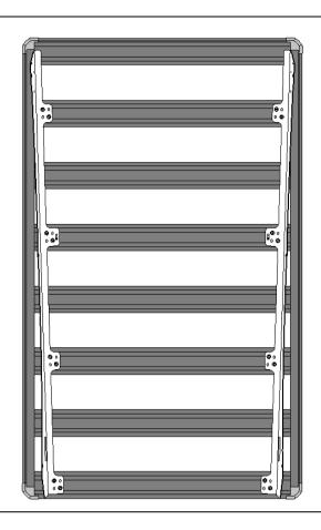
9. Flip the blade brackets over so they are upside down and carefully place on top of the BASE RACK. When doing so ensure the coach bolts in the stud plates go through the slots. Then secure the blade brackets to the BASE RACK using M8 flat washers and nyloc nuts.
