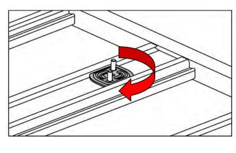
8. Insert the previously assembled stud plates into the correct BASE RACK channels. Rotate the plates 90 degrees.
