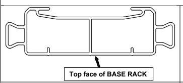
Place the BASE RACK face down on a clean flat surface. Provide protection to the top face of BASE RACK to avoid marking of surfaces
