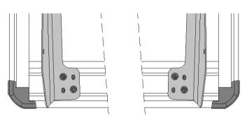
10. Using the previously recorded measurements, adjust the location of the blade bracket on the BASE RACK.
