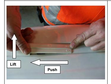
1. Remove the plastic covers from the roof of the vehicle, just the rear four if fitting part No 17920010 or all six if fitting part No 17920010.
