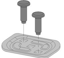
6. Insert 2, M8 x 25 Studs into each of the Stud Plates as shown.
