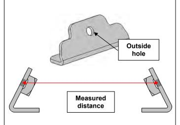
4. Using a tape measure, measure across the vehicle between the middle of the hole on the outside face of the front and rear set of mounting brackets. Make a note of each measurement.
