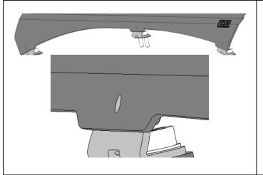
12. With assistance, carefully place the BASE RACK on the vehicle so the inside of the blade brackets rests on the outside of the mounting brackets. The entire BASE RACK assembly should be clear of the vehicle roof. All mounting holes/slots should align closely.
